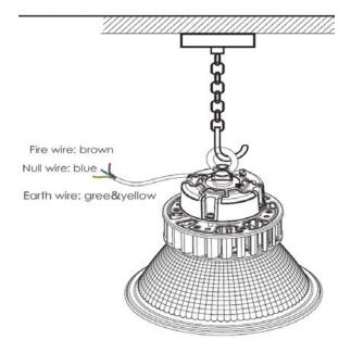
Step 4, Suspend the highbay and make sure not slip off the hook.Wiring and double insulating the cables after lamp well fixed
